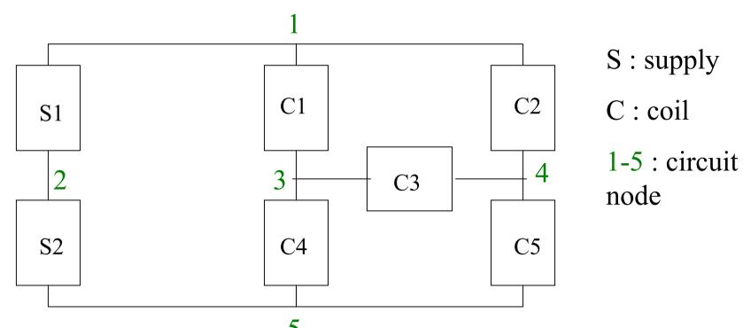
For the given circuit #i above, the connections(i,nnodes(i),2\*ncomponent) matrix reads: S1(1) S1(2) S2(1) S2(2) C1(1) C1(2) C2(1) C2(2) C3(1) C3(2) C4(1) C4(2) C5(1) C5(2)
